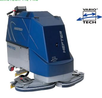
This machine with **VARIOTECH**® technology, automatically operated concerning lifting and lowering to the scrubber head and the work position of the wing. The permanent cleaning width of 112 cm is reducible by pressure to 71 cm. It is pushed back to its original cleaning width by a gas spring.
